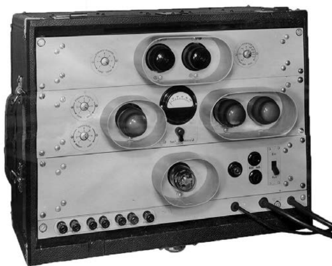
The amplifier set for the HF Magnetophon. From top to bottom: Playback amplifier (V 5), recording amplifier (V 7b), power supply unit (N 7b). The pairs of sockets at the bottom left were probably intended for testing and measuring purposes. © Archive GFGF
