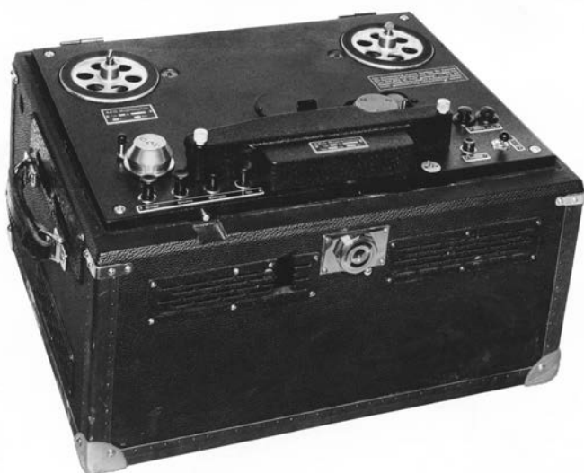
Externally, the drive of the first HF Magnetophon - according to archive documents - is almost identical in construction to the widely used Magnetophon K 4. It probably resembles the version with which the new recording method was presented to the public on 10 June 1941. © Archive GFGF
