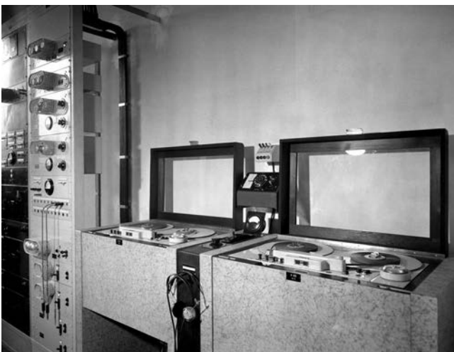
A complete Magnetophon unit of the first radio design, consisting of two R 22 Magnetophons in R 63 chests (front right) and an amplifier rack that accommodated the V 7 amplifiers, among others. - Reichssender Hamburg, the picture is dated 1939.
